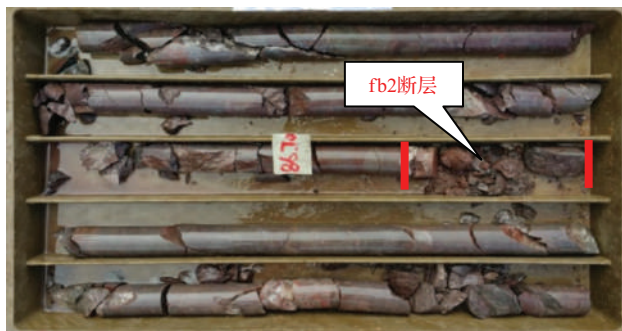
(b) 钻孔揭露断层fb2泥化碎屑带
